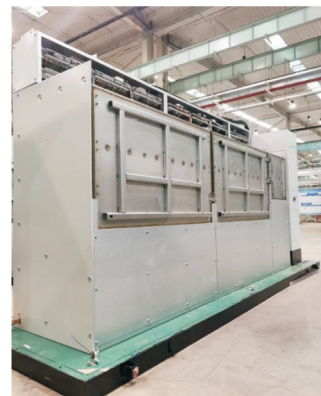
图 13 2.5 mm厚不锈钢钣金焊接气箱实物变形图 Fig. 13 Physical deformation diagram of 2.5 mm-thick stainless steel sheet metal welding gas compartment
